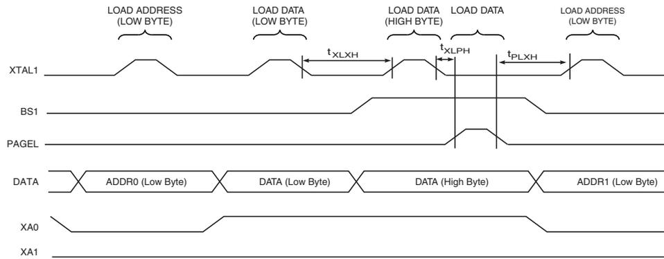
Note: 1. The timing requirements shown in Figure 28-6 (i.e.,  $t_{DVXH}$ ,  $t_{XHXL}$ , and  $t_{XLDX}$ ) also apply to load-ing operation.
