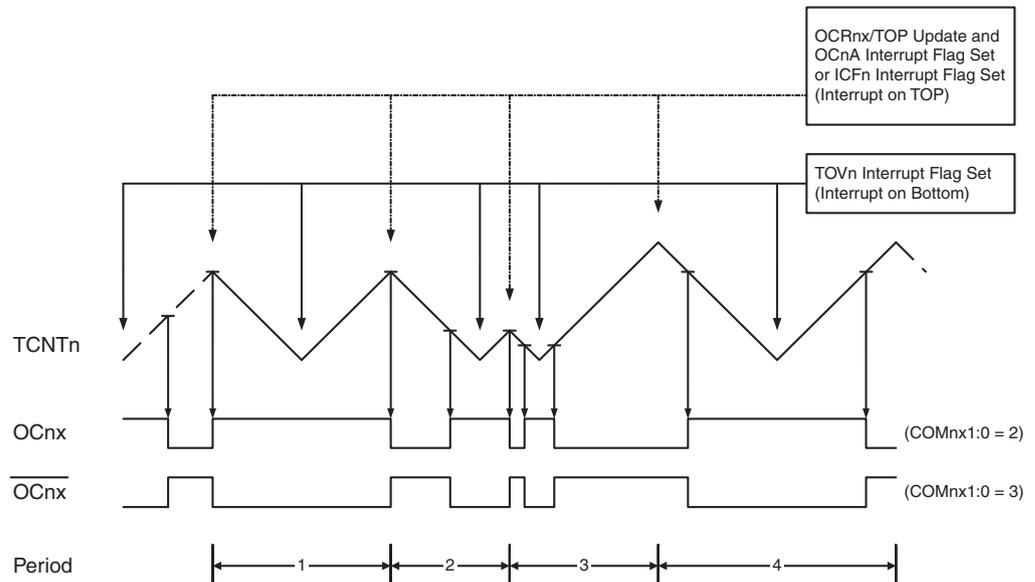
The Timer/Counter Overflow Flag (TOV1) is set each time the counter reaches BOTTOM. When either OCR1A or ICR1 is used for defining the TOP value, the OC1A or ICF1 Flag is set accordingly at the same timer clock cycle as the OCR1x Registers are updated with the double buffer value (at TOP). The Interrupt Flags can be used to generate an interrupt each time the counter reaches the TOP or BOTTOM value.
