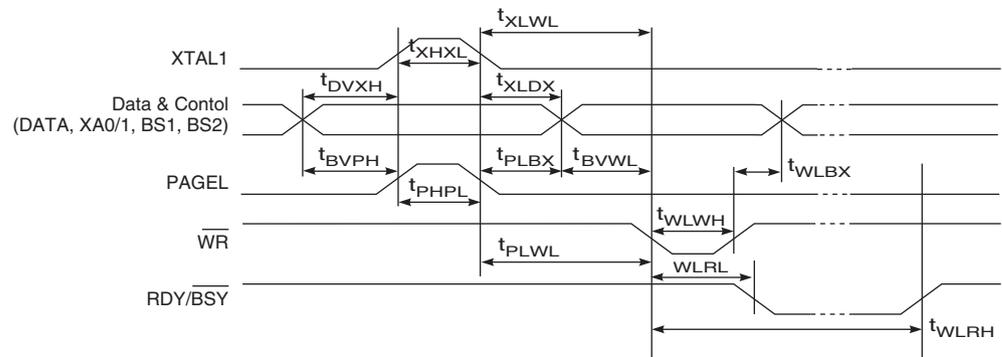
**Figure 28-7. Parallel Programming Timing, Loading Sequence with Timing Requirements<sup>(1)</sup>**
