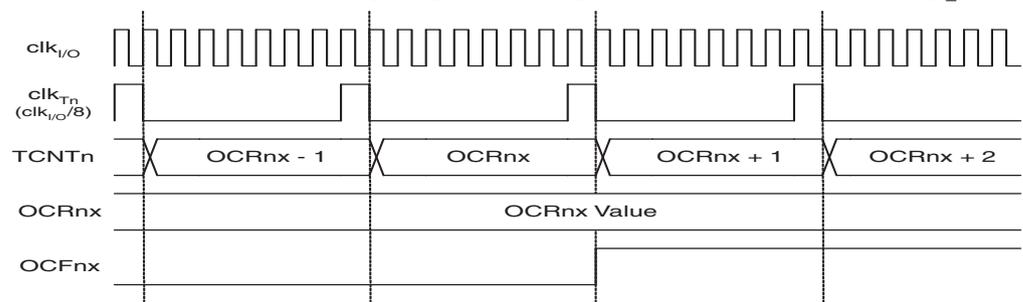
Figure 17-11 shows the setting of OCF2A and the clearing of TCNT2 in CTC mode.
