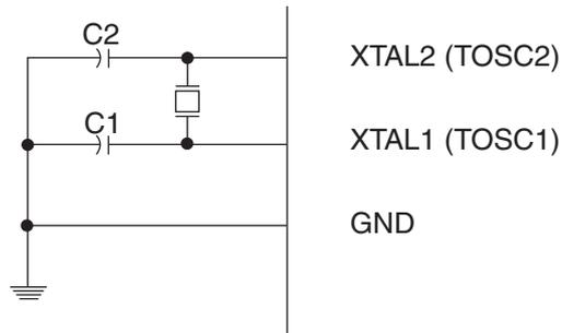
The Low Power Oscillator can operate in three different modes, each optimized for a specific frequency range. The operating mode is selected by the fuses CKSEL3..1 as shown in [Table 8-3 on page 28](#).
