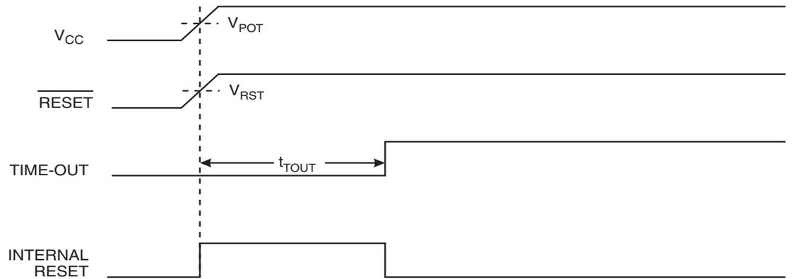
**Figure 10-3.** . MCU Start-up,  $\overline{\text{RESET}}$  Extended Externally
