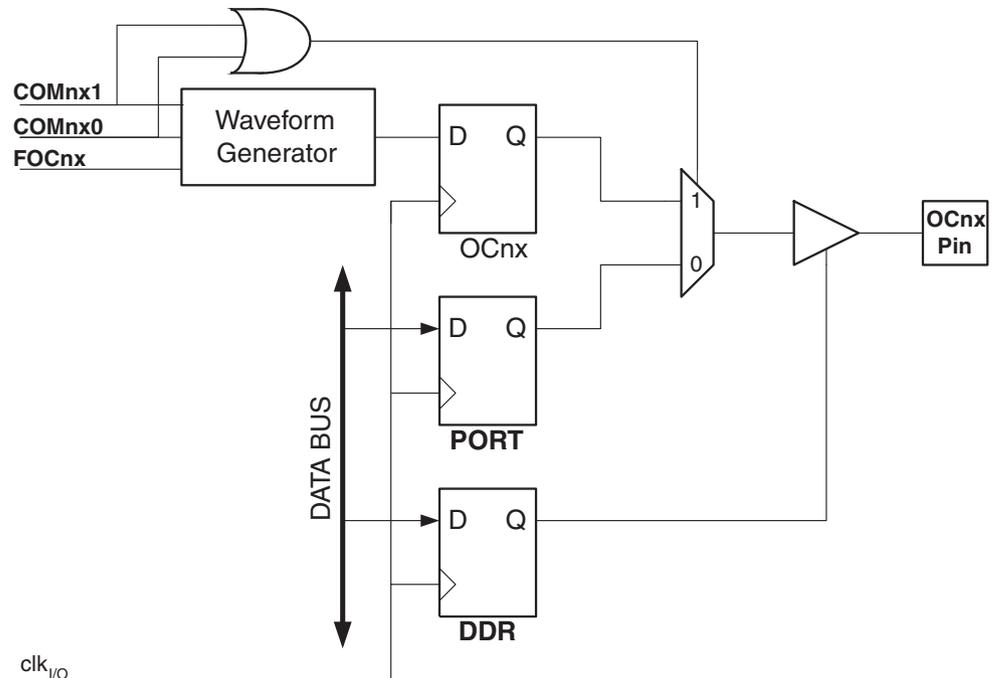
The general I/O port function is overridden by the Output Compare (OC2x) from the Waveform Generator if either of the COM2x1:0 bits are set. However, the OC2x pin direction (input or output) is still controlled by the Data Direction Register (DDR) for the port pin. The Data Direction Register bit for the OC2x pin (DDR\_OC2x) must be set as output before the OC2x value is visible on the pin. The port override function is independent of the Waveform Generation mode.
