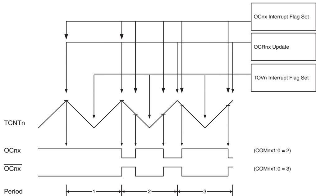
The Timer/Counter Overflow Flag (TOV0) is set each time the counter reaches BOTTOM. The Interrupt Flag can be used to generate an interrupt each time the counter reaches the BOTTOM value.
