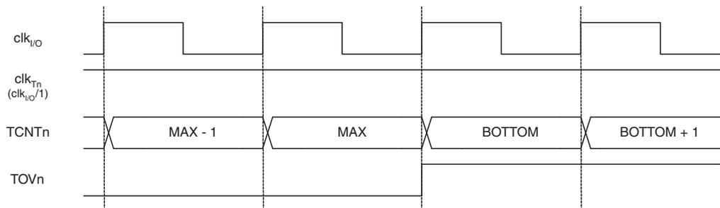
Figure 14-9 shows the same timing data, but with the prescaler enabled.
