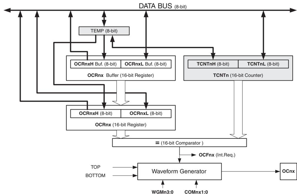
The OCR1x Register is double buffered when using any of the twelve *Pulse Width Modulation* (PWM) modes. For the Normal and *Clear Timer on Compare* (CTC) modes of operation, the double buffering is disabled. The double buffering synchronizes the update of the OCR1x Compare Register to either TOP or BOTTOM of the counting sequence. The synchronization prevents the occurrence of odd-length, non-symmetrical PWM pulses, thereby making the output glitch-free.
