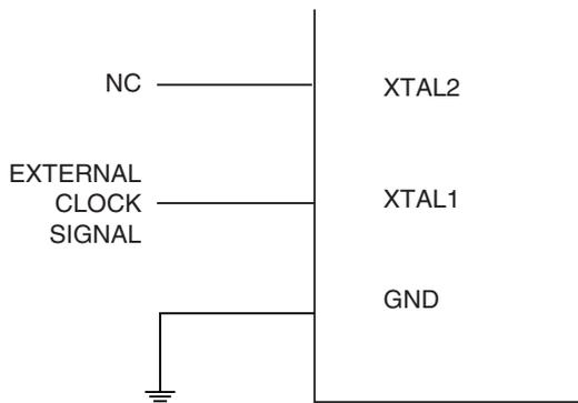
When this clock source is selected, start-up times are determined by the SUT Fuses as shown in [Table 8-15](#).
