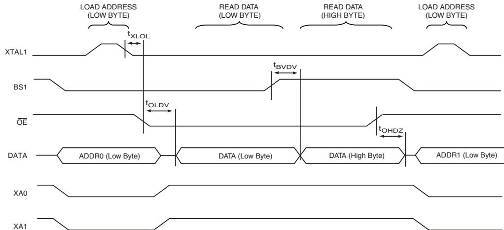
Note: 1. The timing requirements shown in Figure 28-6 (i.e.,  $t_{DVXH}$ ,  $t_{XHXL}$ , and  $t_{XLDX}$ ) also apply to read-ing operation.
