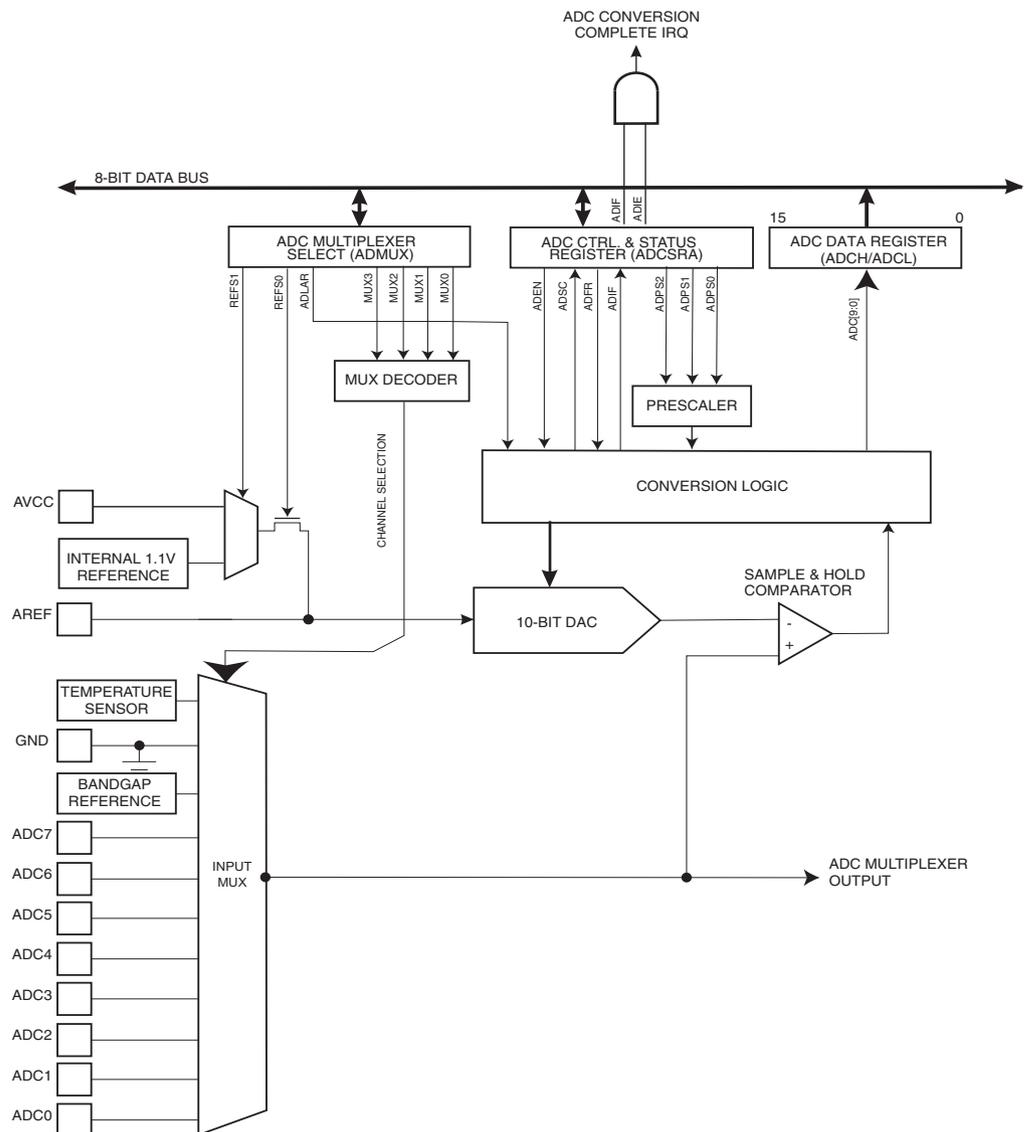
The analog input channel is selected by writing to the MUX bits in ADMUX. Any of the ADC input pins, as well as GND and a fixed bandgap voltage reference, can be selected as single ended inputs to the ADC. The ADC is enabled by setting the ADC Enable bit, ADEN in ADCSRA. Voltage reference and input channel selections will not go into effect until ADEN is set. The ADC does not consume power when ADEN is cleared, so it is recommended to switch off the ADC before entering power saving sleep modes.
